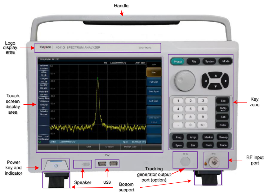
Figure 2.1 Front Panel of 4041 Spectrum Analyzer
